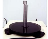
Twist the end of the spindle, so the bottom section is flush with the rest of the spindle.
