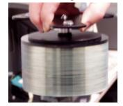
Place the spindle in the front of the duplicator, aligning the arrow with the front of the duplicator. The spindle will lock into place and is ready for use.
